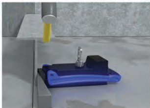
3. Hammer wedge until it pushes piece into place
