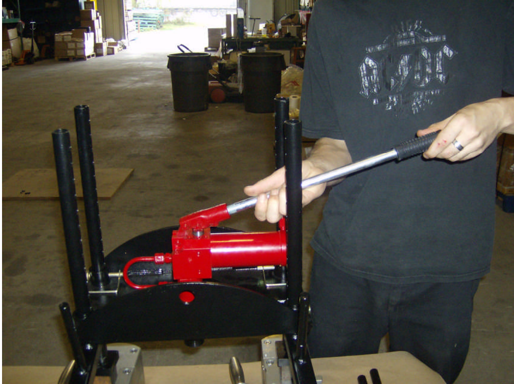
Screw the hydraulic jack handle into the jack.
